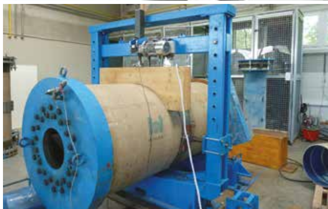
Figures top down: Strain corrosion test, hydrostatic design base (HDB), long-term ring bending test, joint tests.
