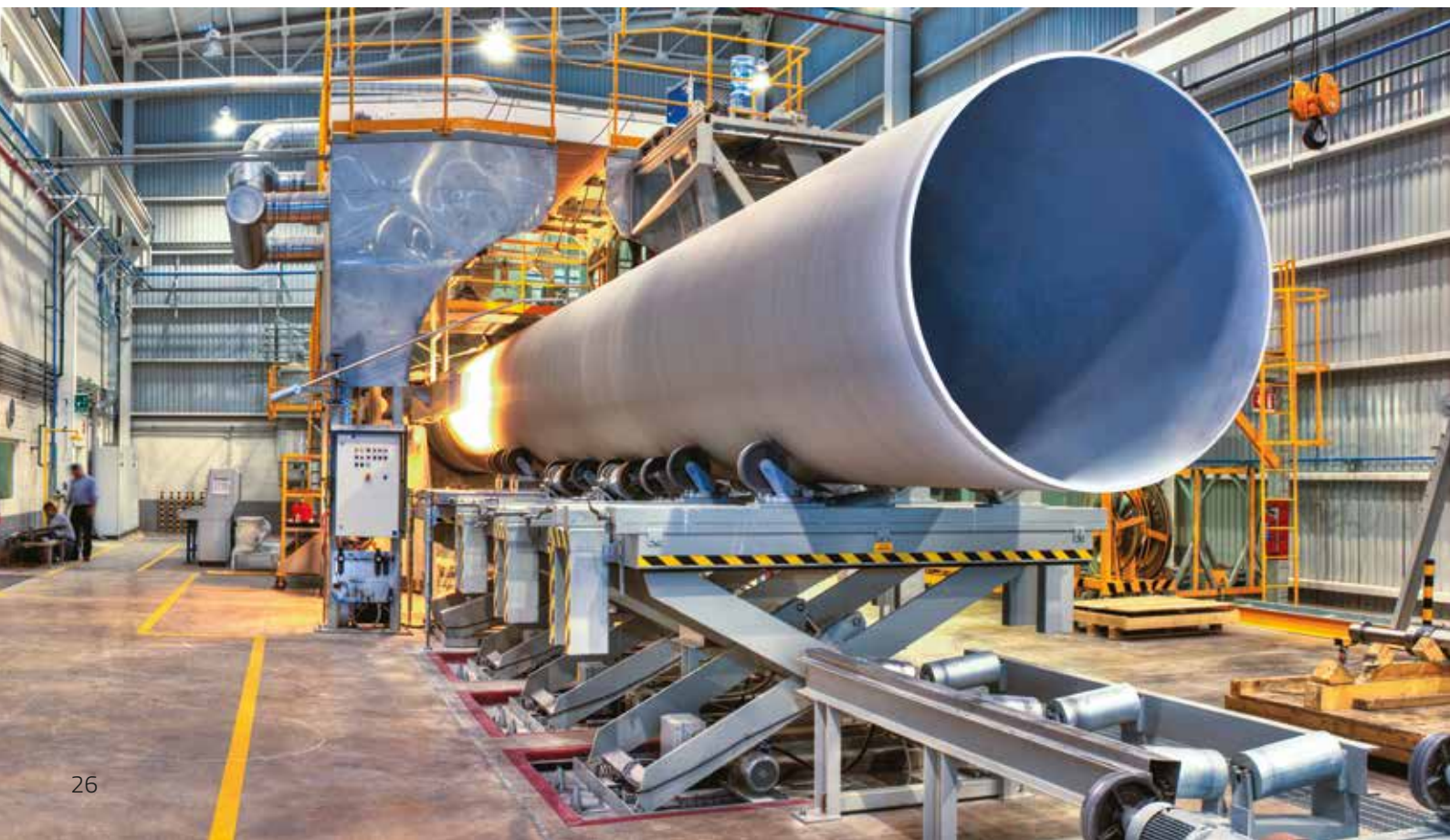
Flowtite pipe produced by continuous filament winding.
