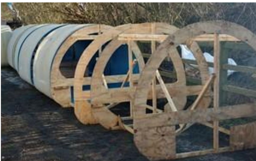
Wooden templates to ensure NC Line profile was manufactured to specification
