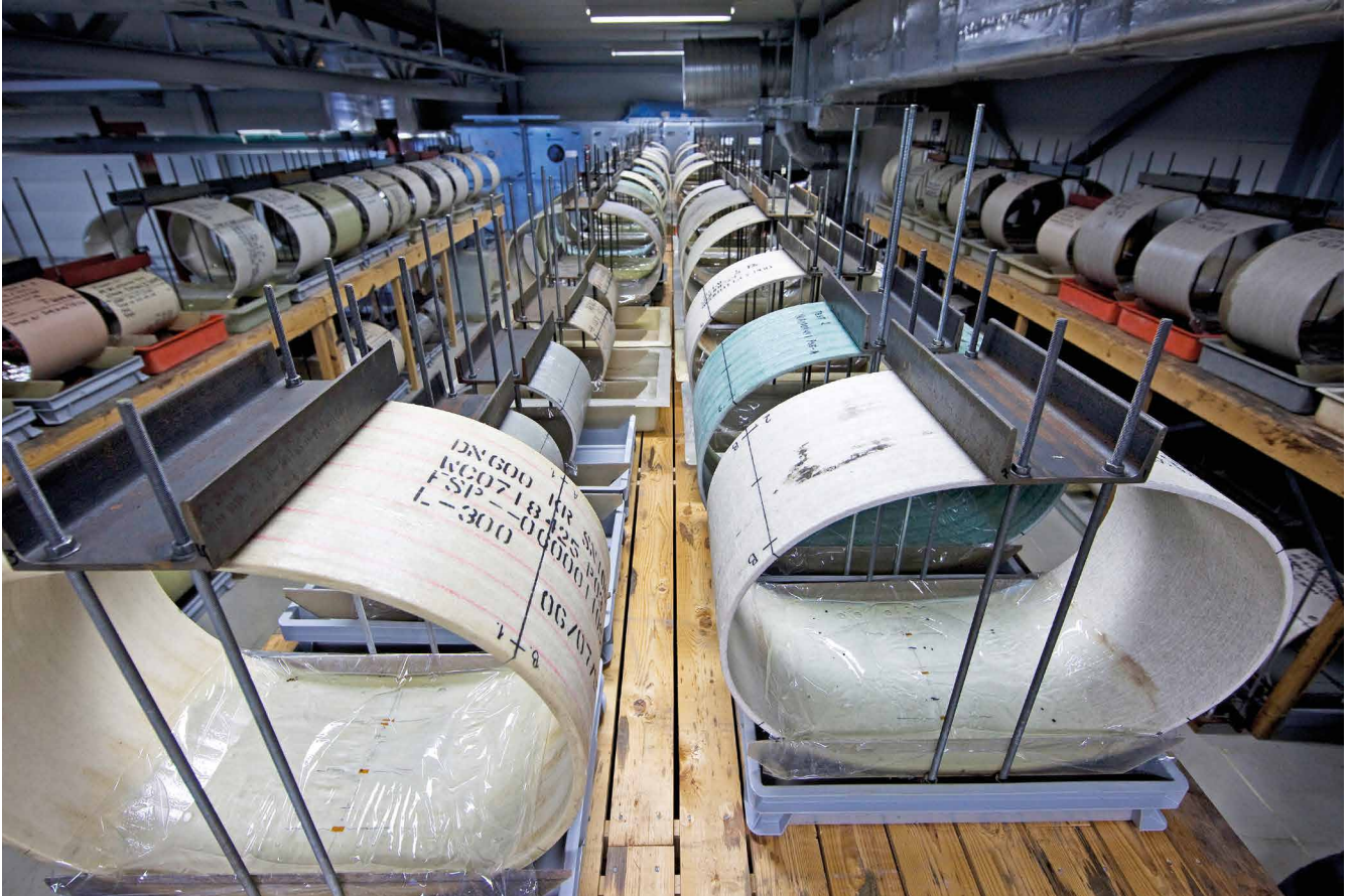
Fig. 1: GRP Long-term corrosion resistance testing since 1978, Amiblu Technology Center in Norway
