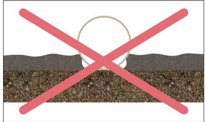
Fig. 14: Improper haunch backfill
