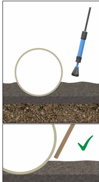
Fig. 15: Proper haunch backfill
