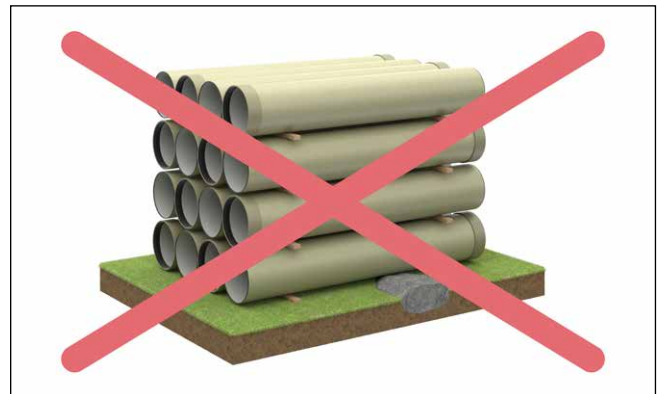
Fig. 8: Pipes should not rest on stones
