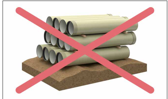
Fig. 9: Pipes should not rest on an uneven surface
