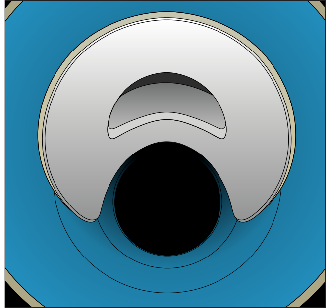
Fig. 60: Lateral connection repair LCR with "Hat Profile"
