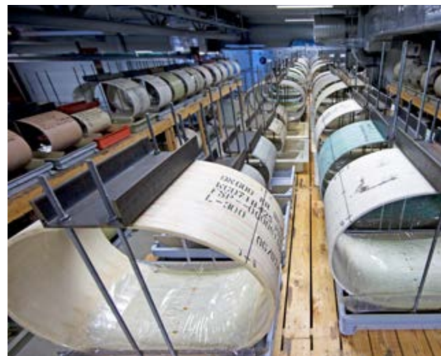
Fig. 1: Strain corrosion tests according to ASTM D3681 in the Amiblu R&D center in Norway.
