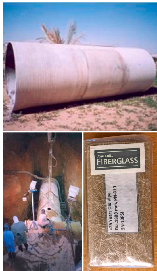
Fig. 9-11: A Flowtite GRP sewer pipe DN 1800 was unearthed and inspected after almost 25 years in service at a sewage treatment plant in Riyadh, SA. The pipe showed no signs of deterioration.
