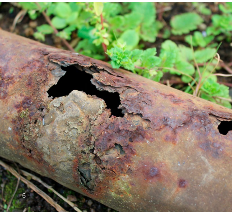
Fig. 1: Pipelines made of concrete or metals corrode in low-pH sewer environments under the influence of sulphuric acid.
