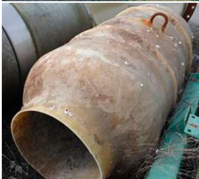
Above: After 33 years of service in seawater, a section of the GRP diffuser was brought ashore to have its mechanical properties tested.
