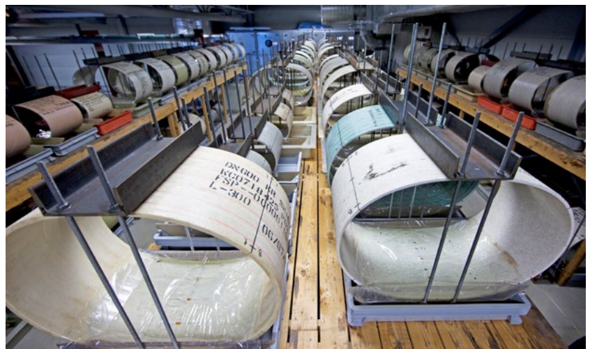
Fig. 4: Strain corrosion tests according to ASTM D3681 in the Amiblu R&D center in Norway.
