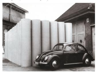
Hoping to find a solution, the owners staged an in-house ideas competition. The rules were that the new material had to allow cylinders of a certain length and specified circular outside diameter to be made, it had to be corrosion resistant, low weight and have a smooth surface in order to ensure uniform dyeing results and also had to be cost effective.
