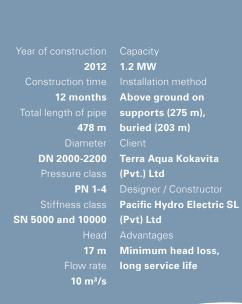
The terrain on site posed quite a few challenges to the installation. It is hilly, made up of partly loose and partly very rocky soil, and the planned pipe route along the Wewa Ganga river bank was very difficult to access. By means of a 20 ton excavator, the pipe sections were transported to their required positions and then installed according to the soil conditions: Roughly half of the 478 m long pipeline was laid on supports above ground (275 m), the other half was buried (203 m).
